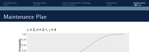
• A plot of the CDF allows system experts to determine if the turnbuckles meet current aircraft standards and when (in some time scale) to perform maintenance on the turnbuckles so pylons will not experience a failure
