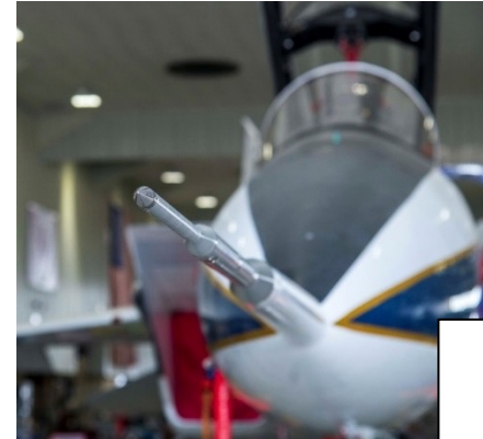
Shock Sensing Probe mounted on NASA F-15
