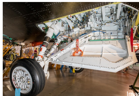
Flight instrumented landing gear installed
